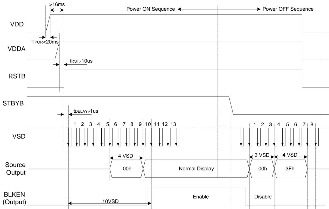
Note: For preventing abnormal operation,  $t_{RST}$  must be longer than 10us during Power ON sequence.
