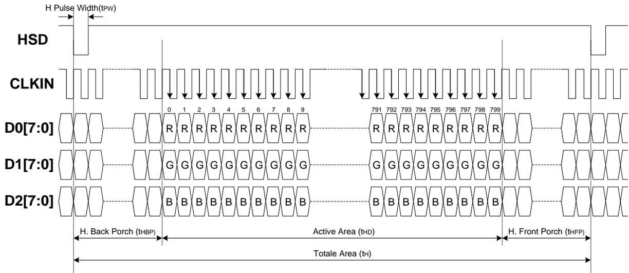
ILI6137A will latch the display data on Dx[7:0] bus at rising edge of CLKIN when CLKPOL is set to “H”, the input data timing is illustrated as below:
