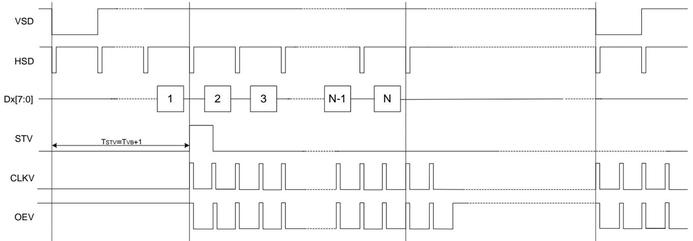
**Vertical Timing Diagram of DE Mode (Dual Gate)**
