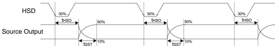
**Vertical Timing Diagram of SYNC Mode (Dual Gate)**
