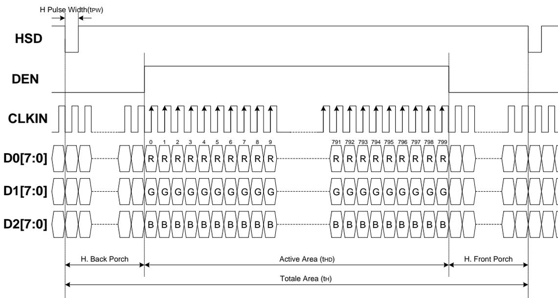
ILI6137A will latch the display data on Dx[7:0] bus at falling edge of CLKIN when CLKPOL is set to “L”, the input data timing is illustrated as below:
